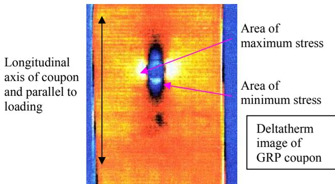
Note that the stress directly above and below the hole is less than the nominal stress, however this is only a localised effect and diminishes with distance from the defect as the matrix redistributes load to fibres bisected by the hole. Effects like this are understood and can be modelled however this must be done early in the design process and details that are likely to cause stress concentrations should not be grouped together as they will have a cumulative effect in weakening the structure.
